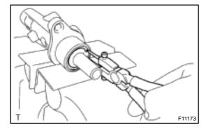
(b) Using snap ring pliers, install the snap ring.
